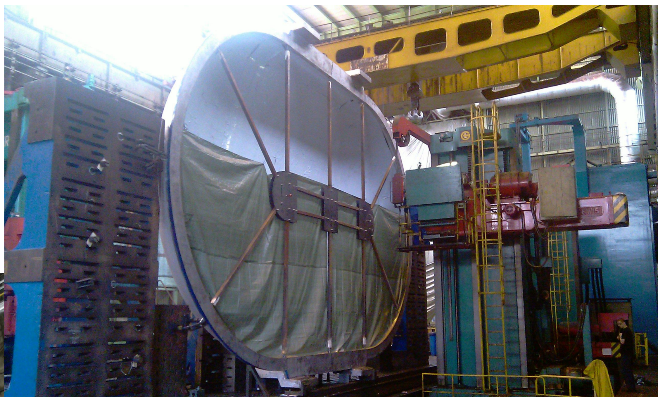
Machining of the main flange (see scale with operator on right)
